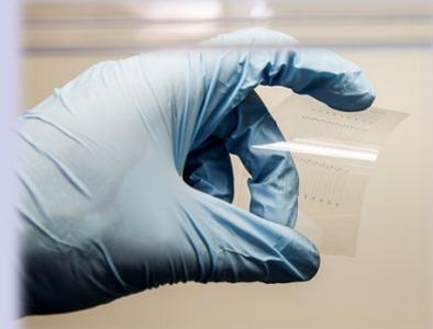
**Fig. 1.** All-polymer, fully printed logic circuits @IIT.
